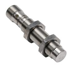
Contrinex inductive proximity sensor, tubular, 12mm diameter x 60mm, 304 stainless steel housing, NPN, N.O., 3mm sensing distance, non-flush, 400 Hz switching frequency, IP68 IP69K, 4-pin M12 quick-disconnect.
