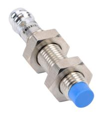
Contrinex inductive proximity sensor, tubular, 8mm diameter x 45mm body, 304 stainless steel housing, PNP, N.C. output, 4mm sensing distance, non-flush, 3.5 kHz switching frequency, IP67, 3-pin M8 quick-disconnect.
