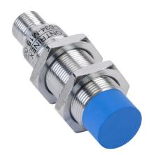
Contrinex inductive proximity sensor, tubular, 18mm diameter x 63.5mm body, nickel-plated brass housing, PNP, N.C. output, 12mm sensing distance, non-flush, 500 Hz switching frequency, IP67, 4-pin M12 quick-disconnect.
