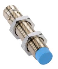
Contrinex inductive proximity sensor, tubular, 12mm diameter x 60mm body, nickel-plated brass housing, PNP, N.C. output, 8mm sensing distance, non-flush, 1.4 kHz switching frequency, IP67, 4-pin M12 quick-disconnect.
