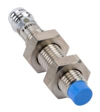
Contrinex inductive proximity sensor, tubular, 8mm diameter x 45mm body, 304 stainless steel housing, PNP, N.O. output, 4mm sensing distance, non-flush, 3.5 kHz switching frequency, IP67, 3-pin M8 quick-disconnect.
