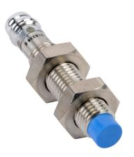
Contrinex inductive proximity sensor, tubular, 8mm diameter x 45mm body, 304 stainless steel housing, PNP, N.O. output, 4mm sensing distance, non-flush, 3.5 kHz switching frequency, IP67, 3-pin M8 quick-disconnect.
