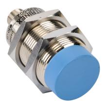
Contrinex inductive proximity sensor, tubular, 30mm diameter x 63.5mm body, nickel-plated brass housing, PNP, N.O. output, 25mm sensing distance, non-flush, 200 Hz switching frequency, IP67, 4-pin M12 quick-disconnect.
