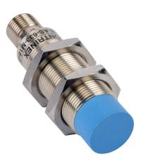
Contrinex inductive proximity sensor, tubular, 18mm diameter x 63.5mm body, nickel-plated brass housing, PNP, N.O. output, 12mm sensing distance, non-flush, 500 Hz switching frequency, IP67, 4-pin M12 quick-disconnect.
