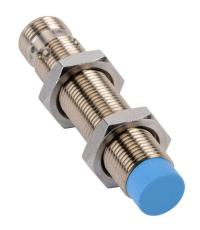
Contrinex inductive proximity sensor, tubular, 12mm diameter x 60mm body, nickel-plated brass housing, PNP, N.O. output, 8mm sensing distance, non-flush, 1.4 kHz switching frequency, IP67, 4-pin M12 quick-disconnect.
