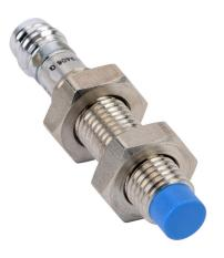
Contrinex inductive proximity sensor, tubular, 8mm diameter x 45mm body, 304 stainless steel housing, NPN, N.O. output, 4mm sensing distance, non-flush, 3.5 kHz switching frequency, IP67, 3-pin M8 quick-disconnect.
