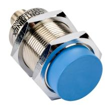
Contrinex inductive proximity sensor, tubular, 30mm diameter x 63.5mm body, nickel-plated brass housing, NPN, N.O. output, 25mm sensing distance, non-flush, 200 Hz switching frequency, IP67, 4-pin M12 quick-disconnect.
