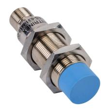
Contrinex inductive proximity sensor, tubular, 18mm diameter x 63.5mm body, nickel-plated brass housing, NPN, N.O. output, 12mm sensing distance, non-flush, 500 Hz switching frequency, IP67, 4-pin M12 quick-disconnect.
