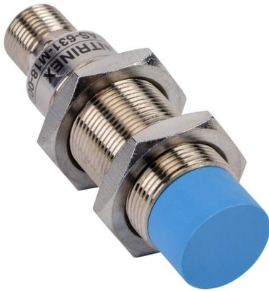
Contrinex inductive proximity sensor, tubular, 18mm diameter x 63.5mm body, nickel-plated brass housing, NPN, N.O. output, 12mm sensing distance, non-flush, 500 Hz switching frequency, IP67, 4-pin M12 quick-disconnect.
