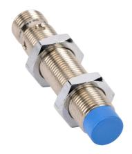
Contrinex inductive proximity sensor, tubular, 12mm diameter x 60mm body, nickel-plated brass housing, NPN, N.O. output, 8mm sensing distance, non-flush, 1.4 kHz switching frequency, IP67, 4-pin M12 quick-disconnect.
