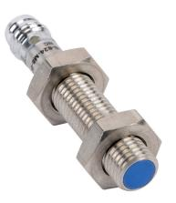
Contrinex inductive proximity sensor, tubular, 8mm diameter x 35mm body, 304 stainless steel housing, PNP, N.C. output, 2mm sensing distance, flush, 5 kHz switching frequency, IP67, 3-pin M8 quick-disconnect.
