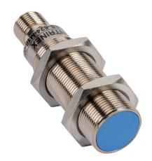
Contrinex inductive proximity sensor, tubular, 18mm diameter x 63.5mm body, nickel-plated brass housing, PNP, N.C. output, 8mm sensing distance, flush, 1.5 kHz switching frequency, IP67, 4-pin M12 quick-disconnect.
