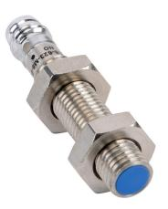
Contrinex inductive proximity sensor, tubular, 8mm diameter x 35mm body, 304 stainless steel housing, PNP, N.O. output, 2mm sensing distance, flush, 5 kHz switching frequency, IP67, 3-pin M8 quick-disconnect.
