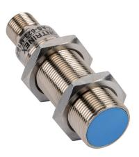
Contrinex inductive proximity sensor, tubular, 18mm diameter x 63.5mm body, nickel-plated brass housing, PNP, N.O. output, 8mm sensing distance, flush, 1.5 kHz switching frequency, IP67, 4-pin M12 quick-disconnect.
