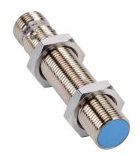
Contrinex inductive proximity sensor, tubular, 12mm diameter x 60mm body, nickel-plated brass housing, PNP, N.O. output, 4mm sensing distance, flush, 2.5 kHz switching frequency, IP67, 4-pin M12 quick-disconnect.
