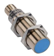
Contrinex inductive proximity sensor, tubular, 18mm diameter x 63.5mm body, nickel-plated brass housing, NPN, N.O. output, 8mm sensing distance, flush, 1.5 kHz switching frequency, IP67, 4-pin M12 quick-disconnect.
