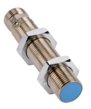
Contrinex inductive proximity sensor, tubular, 12mm diameter x 60mm body, nickel-plated brass housing, NPN, N.O. output, 4mm sensing distance, flush, 2.5 kHz switching frequency, IP67, 4-pin M12 quick-disconnect.
