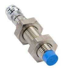
Contrinex inductive proximity sensor, tubular, 8mm diameter x 45mm body, 304 stainless steel housing, PNP, N.C. output, 2.5mm sensing distance, non-flush, 4.5 kHz switching frequency, IP67, 3-pin M8 quick-disconnect.
