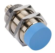
Contrinex inductive proximity sensor, tubular, 30mm diameter x 63.5mm body, nickel-plated brass housing, PNP, N.C. output, 15mm sensing distance, non-flush, 700 Hz switching frequency, IP67, 4-pin M12 quick-disconnect.
