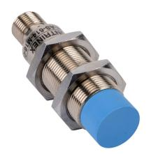
Contrinex inductive proximity sensor, tubular, 18mm diameter x 63.5mm body, nickel-plated brass housing, PNP, N.C. output, 8mm sensing distance, non-flush, 2 kHz switching frequency, IP67, 4-pin M12 quick-disconnect.
