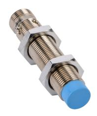
Contrinex inductive proximity sensor, tubular, 12mm diameter x 60mm body, nickel-plated brass housing, PNP, N.C. output, 4mm sensing distance, non-flush, 2 kHz switching frequency, IP67, 4-pin M12 quick-disconnect.
