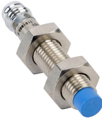
Contrinex inductive proximity sensor, tubular, 8mm diameter x 45mm body, 304 stainless steel housing, PNP, N.O. output, 2.5mm sensing distance, non-flush, 4.5 kHz switching frequency, IP67, 3-pin M8 quick-disconnect.
