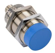
Contrinex inductive proximity sensor, tubular, 30mm diameter x 63.5mm body, nickel-plated brass housing, PNP, N.O. output, 15mm sensing distance, non-flush, 700 Hz switching frequency, IP67, 4-pin M12 quick-disconnect.
