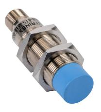
Contrinex inductive proximity sensor, tubular, 18mm diameter x 63.5mm body, nickel-plated brass housing, PNP, N.O. output, 8mm sensing distance, non-flush, 2 kHz switching frequency, IP67, 4-pin M12 quick-disconnect.
