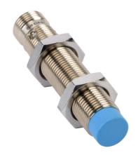
Contrinex inductive proximity sensor, tubular, 12mm diameter x 60mm body, nickel-plated brass housing, PNP, N.O. output, 4mm sensing distance, non-flush, 2 kHz switching frequency, IP67, 4-pin M12 quick-disconnect.
