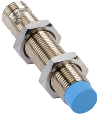
Contrinex inductive proximity sensor, tubular, 12mm diameter x 60mm body, nickel-plated brass housing, PNP, N.O. output, 4mm sensing distance, non-flush, 2 kHz switching frequency, IP67, 4-pin M12 quick-disconnect.
