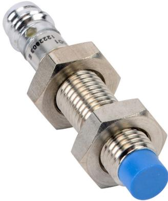
Contrinex inductive proximity sensor, tubular, 8mm diameter x 45mm body, 304 stainless steel housing, NPN, N.O. output, 2.5mm sensing distance, non-flush, 4.5 kHz switching frequency, IP67, 3-pin M8 quick-disconnect.
