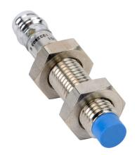
Contrinex inductive proximity sensor, tubular, 8mm diameter x 45mm body, 304 stainless steel housing, NPN, N.O. output, 2.5mm sensing distance, non-flush, 4.5 kHz switching frequency, IP67, 3-pin M8 quick-disconnect.
