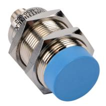
Contrinex inductive proximity sensor, tubular, 30mm diameter x 63.5mm body, nickel-plated brass housing, NPN, N.O. output, 15mm sensing distance, non-flush, 700 Hz switching frequency, IP67, 4-pin M12 quick-disconnect.
