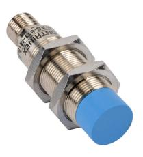
Contrinex inductive proximity sensor, tubular, 18mm diameter x 63.5mm body, nickel-plated brass housing, NPN, N.O. output, 8mm sensing distance, non-flush, 2 kHz switching frequency, IP67, 4-pin M12 quick-disconnect.
