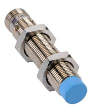
Contrinex inductive proximity sensor, tubular, 12mm diameter x 60mm body, nickel-plated brass housing, NPN, N.O. output, 4mm sensing distance, non-flush, 2 kHz switching frequency, IP67, 4-pin M12 quick-disconnect.
