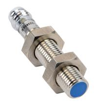
Contrinex inductive proximity sensor, tubular, 8mm diameter x 45mm body, 304 stainless steel housing, PNP, N.C. output, 1.5mm sensing distance, flush, 5 kHz switching frequency, IP67, 3-pin M8 quick-disconnect.
