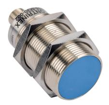
Contrinex inductive proximity sensor, tubular, 30mm diameter x 63.5mm body, nickel-plated brass housing, PNP, N.C. output, 10mm sensing distance, flush, 1.2 kHz switching frequency, IP67, 4-pin M12 quick-disconnect.
