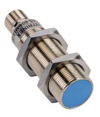
Contrinex inductive proximity sensor, tubular, 18mm diameter x 63.5mm body, nickel-plated brass housing, PNP, N.C. output, 5mm sensing distance, flush, 2 kHz switching frequency, IP67, 4-pin M12 quick-disconnect.
