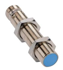
Contrinex inductive proximity sensor, tubular, 12mm diameter x 60mm body, nickel-plated brass housing, PNP, N.C. output, 2mm sensing distance, flush, 3 kHz switching frequency, IP67, 4-pin M12 quick-disconnect.
