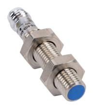
Contrinex inductive proximity sensor, tubular, 8mm diameter x 45mm body, 304 stainless steel housing, PNP, N.O. output, 1.5mm sensing distance, flush, 5 kHz switching frequency, IP67, 3-pin M8 quick-disconnect.
