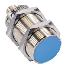
Contrinex inductive proximity sensor, tubular, 30mm diameter x 63.5mm body, nickel-plated brass housing, PNP, N.O. output, 10mm sensing distance, flush, 1.2 kHz switching frequency, IP67, 4-pin M12 quick-disconnect.
