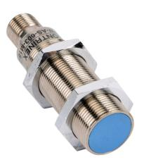
Contrinex inductive proximity sensor, tubular, 18mm diameter x 63.5mm body, nickel-plated brass housing, PNP, N.O. output, 5mm sensing distance, flush, 2 kHz switching frequency, IP67, 4-pin M12 quick-disconnect.
