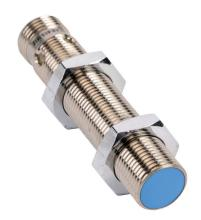
Contrinex inductive proximity sensor, tubular, 12mm diameter x 60mm body, nickel-plated brass housing, PNP, N.O. output, 2mm sensing distance, flush, 3 kHz switching frequency, IP67, 4-pin M12 quick-disconnect.
