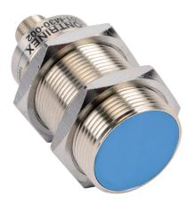
Contrinex inductive proximity sensor, tubular, 30mm diameter x 63.5mm body, nickel-plated brass housing, NPN, N.O. output, 10mm sensing distance, flush, 1.2 kHz switching frequency, IP67, 4-pin M12 quick-disconnect.
