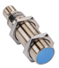
Contrinex inductive proximity sensor, tubular, 18mm diameter x 63.5mm body, nickel-plated brass housing, NPN, N.O. output, 5mm sensing distance, flush, 2 kHz switching frequency, IP67, 4-pin M12 quick-disconnect.
