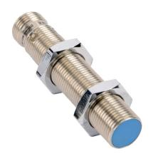
Contrinex inductive proximity sensor, tubular, 12mm diameter x 60mm body, nickel-plated brass housing, NPN, N.O. output, 2mm sensing distance, flush, 3 kHz switching frequency, IP67, 4-pin M12 quick-disconnect.
