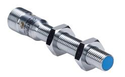
Contrinex inductive proximity sensor, tubular, 8mm diameter x 66mm body, chrome-plated nickel silver housing, PNP, N.C. output, 4mm sensing distance, semi-flush, 500 Hz switching frequency, IP67, 4-pin M12 quick-disconnect.
