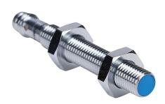
Contrinex inductive proximity sensor, tubular, 8mm diameter x 60mm body, chrome-plated nickel silver housing, PNP, N.C. output, 4mm sensing distance, semi-flush, 500 Hz switching frequency, IP67, 3-pin M8 quick-disconnect.
