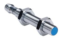
Contrinex inductive proximity sensor, tubular, 8mm diameter x 60mm body, chrome-plated nickel silver housing, PNP, N.C. output, 4mm sensing distance, semi-flush, 500 Hz switching frequency, IP67, 3-pin M8 quick-disconnect.
