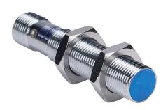
Contrinex inductive proximity sensor, tubular, 12mm diameter x 60mm body, chrome-plated brass housing, PNP, N.C. output, 8mm sensing distance, semi-flush, 400 Hz switching frequency, IP67, 4-pin M12 quick-disconnect.
