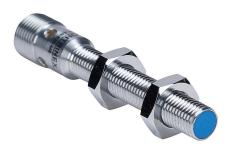
Contrinex inductive proximity sensor, tubular, 8mm diameter x 66mm body, chrome-plated nickel silver housing, PNP, N.O. output, 4mm sensing distance, semi-flush, 500 Hz switching frequency, IP67, 4-pin M12 quick-disconnect.
