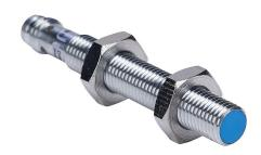
Contrinex inductive proximity sensor, tubular, 8mm diameter x 60mm body, chrome-plated nickel silver housing, PNP, N.O. output, 4mm sensing distance, semi-flush, 500 Hz switching frequency, IP67, 3-pin M8 quick-disconnect.
