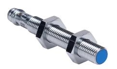
Contrinex inductive proximity sensor, tubular, 8mm diameter x 60mm body, chrome-plated nickel silver housing, NPN, N.C. output, 4mm sensing distance, semi-flush, 500 Hz switching frequency, IP67, 3-pin M8 quick-disconnect.
