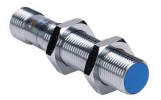
Contrinex inductive proximity sensor, tubular, 12mm diameter x 60mm body, chrome-plated brass housing, NPN, N.C. output, 8mm sensing distance, semi-flush, 400 Hz switching frequency, IP67, 4-pin M12 quick-disconnect.
