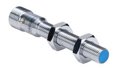
Contrinex inductive proximity sensor, tubular, 8mm diameter x 66mm body, chrome-plated nickel silver housing, NPN, N.O. output, 4mm sensing distance, semi-flush, 500 Hz switching frequency, IP67, 4-pin M12 quick-disconnect.
